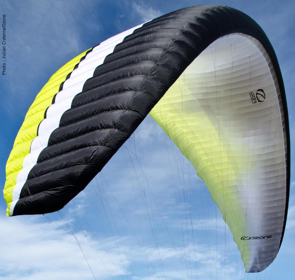
Another effect of the Sharknose is that the air intakes are set back and as a consequence, this completely closes the nose, increasing the efficiency of this part of the profile. The nose bites at the air better.
